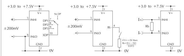
Measuring a single ended input voltage referenced to supply, i.e. the input voltage and the meter's power supply share the same 0V rail. Ensure solder link LCOM is open.
